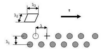
Figure 1. A schematic illustration of a transition of a molecular-kinetic unit in a liquid from one stable position to another (H. Eyring [1]).
