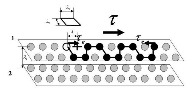
Figure 2. A schematic illustration of a transition of a molecular-kinetic unit of a stretched polymeric chain into a new equilibrium position during the flow of two layers of the liquid with different rates with respect to each other
