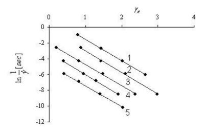
Figure 3. Logarithm of the inverse shear rate vs. high-elastic deformations of polyisobutylene at steady-state flow regimes. Temperatures, °C: 1-22; 2-40; 3-60; 4-80; 5-100. (Data recalculated from Ref. [16]).
